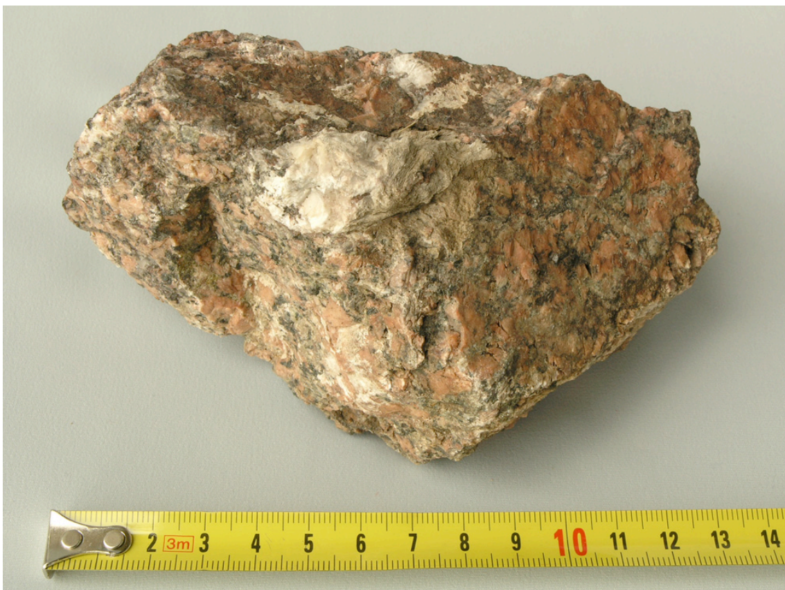
Fig.1 Inclusions of massive calcite in granite at three sites. Largest piece in centre, smaller pieces far up and far down.
